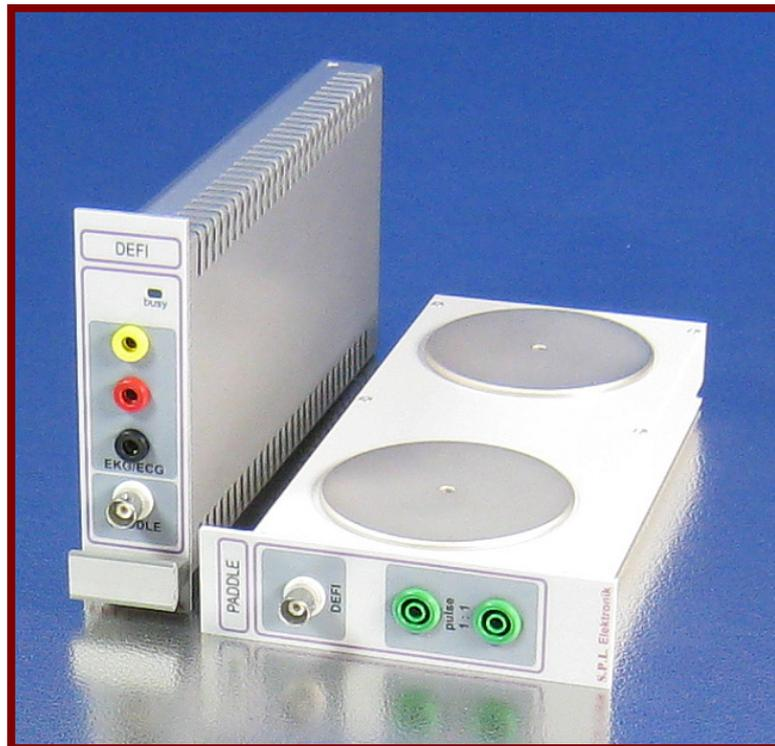
**The GS Testing Module for function tests of external defibrillators in accordance to IEC 60601-2-4**
